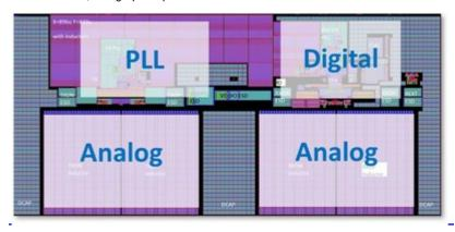
Samsung's 2nm process is its third generation of gate-all-around (GAA) process technologies and continues the rapid progression of Moore's Law using novel transistor devices for higher integration density, faster performance, and lower power. RedHawk-SC provides industry-recognized signoff verification for electromigration (EM) and voltage drop (IR drop) on power distribution networks for digital designs. Totem provides similar checking for custom analog and mixed-signal designs.
