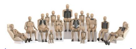
Humanetics is the world's leading provider of anthropomorphic test devices (ATDs), more commonly known as crash test dummies. The company also provides digital models of their ATDs, which are commonly used by simulation software companies, including Ansys, to create realistic simulations of crash events. Humanetics' digital models of ATDs are highly complementary to, and frequently used with Ansys' LS-DYNA crash test solution.
