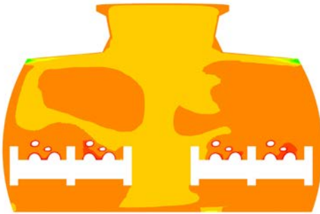
▲ Detailed ANSYS CFD predictions of temperature within the cabin during the initial taxiing stage of a simulated flight on a hot day
