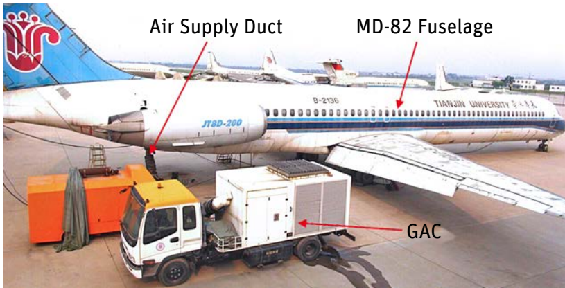
▲ The MD-82 aircraft and GAC system used to heat or cool the cabin on the ground
