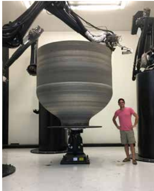
Relativity's Stargate is the world's largest 3D printer.
