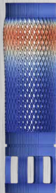
ANSYS additive manufacturing simulation of the original design matched the distortion shown on the real part.
