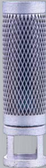
A combination of supports and distortion compensation made it possible to eliminate the distortion problem.
