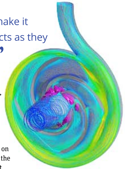
▲ A 3-D simulation model shows that cavitation, as visualized by the purple vapor bubbles, is the effect of a faulty valve and the cause of a vibration problem.
