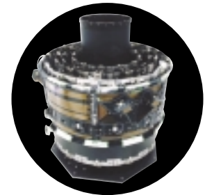
NASA Chandra X-ray Telescope high resolution mirror system "support structure assembly."
