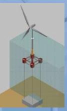
Design of floating offshore wind turbine
