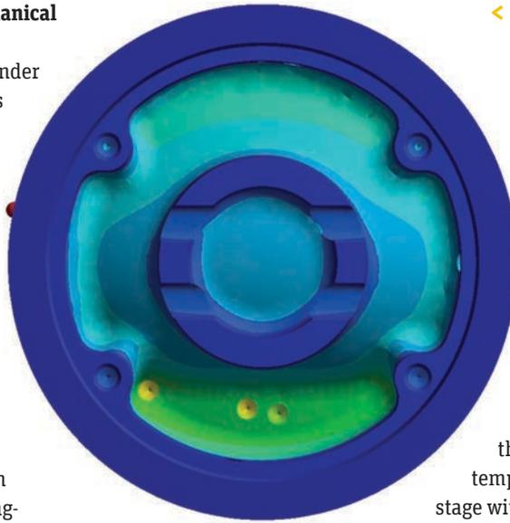
◀ Temperatures under the crown of the piston as predicted by advanced piston thermal modeling
