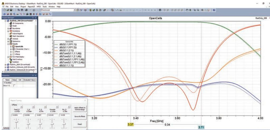
Derivative tuning allows fine adjustments without the need for additional simulation runs.
