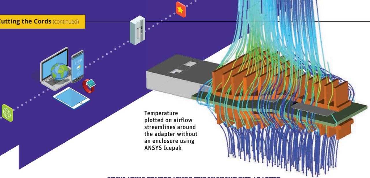
Temperature plotted on airflow streamlines around the adapter without an enclosure using ANSYS Icepak
