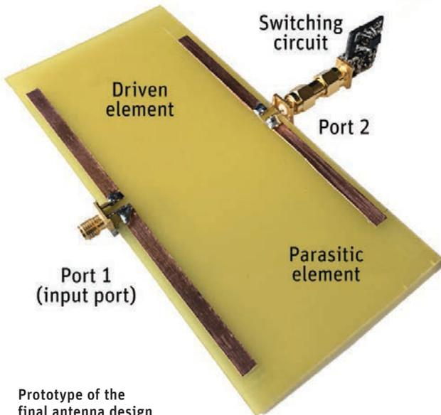
Prototype of the final antenna design
