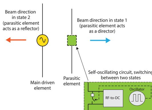
Schematic of new reconfigurable antenna design
