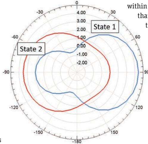
Simulated antenna radiation pattern with radial axis representing realized gain at 900 MHz in YZ plane
