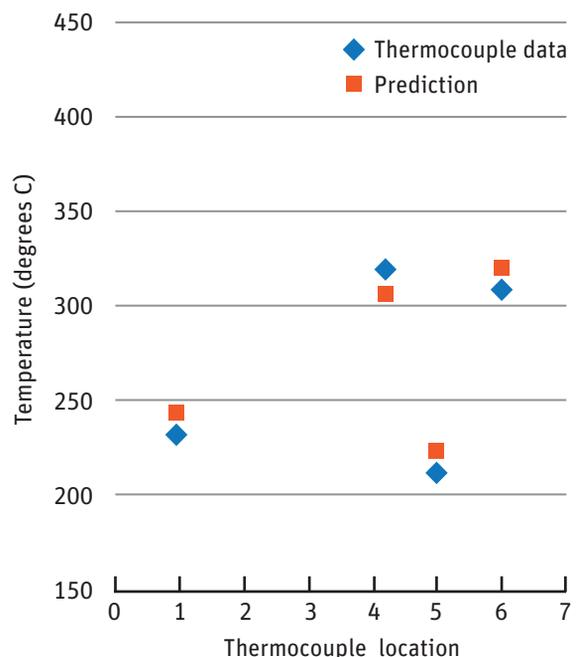
Piston temperatures as predicted by advanced thermal modeling correlate well with thermocouple measurements.
