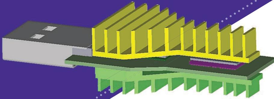
◀ ANSYS Icepak model of interior components of the adapter shows: top heatsink (yellow) connected to 115 C-rated components, bottom heatsink (light green) connected to PCB, one of 115 C-rated components (red), PCB (green) and USB connector (gray).
